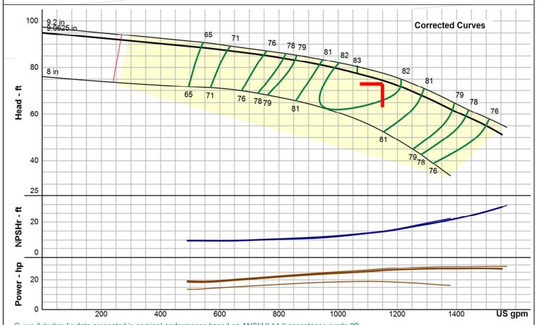
Curve & hydraulic data presented is nominal performance based on ANSI/HI 14.6 acceptance grade 2B. Design values are guaranteed within the following tolerances: Flow  $\pm$  8%, Head  $\pm$  5%, and optionally either Power + 8% or Efficiency - 5% at manufacturer's discretion.
