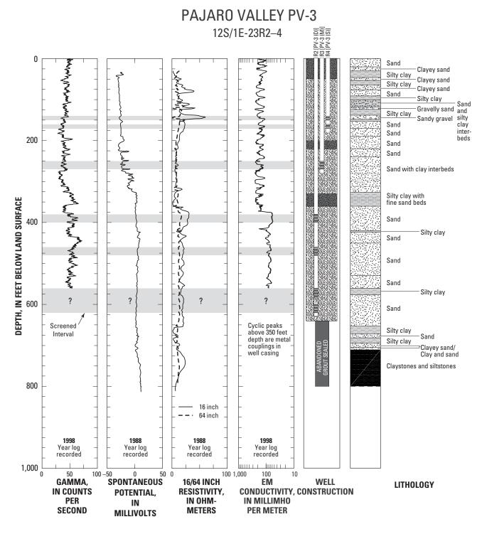
Figure A1.2. Geophysical logs and well construction for selected monitoring wells and test holes in the Pajaro Valley, Santa Cruz County, California.
