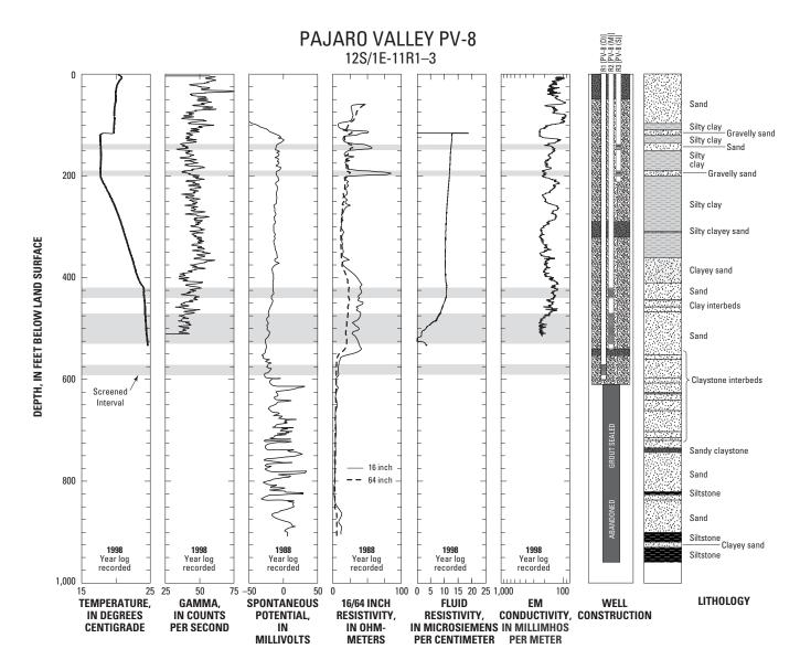
Figure A1.6. Geophysical logs and well construction for selected monitoring wells and test holes in the Pajaro Valley, Santa Cruz County, California.
