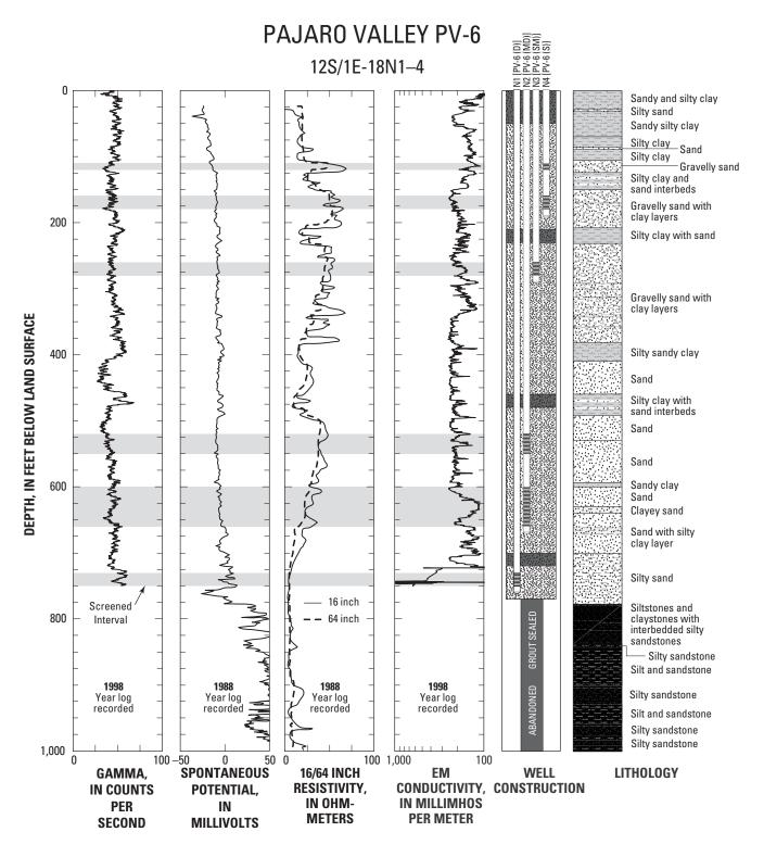
Figure A1.5. Geophysical logs and well construction for selected monitoring wells and test holes in the Pajaro Valley, Santa Cruz County, California.
