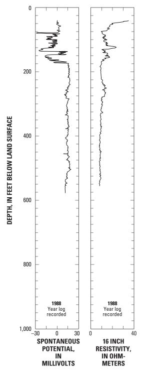
**Figure A1.4.** Geophysical logs for selected monitoring wells and test holes in the Pajaro Valley, Monterey County, California.
