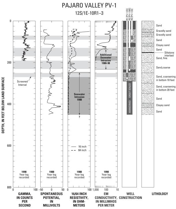
**Figure A1.1.** Geophysical logs and well construction for selected monitoring wells and test holes in the Pajaro Valley, Santa Cruz County, California.
